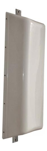
*Single bay* broadband four dipole panel covering the 470-698 MHz spectrum. The radiating elements and structural dipoles are entirely welded to the support spine. This results in an enhanced reduction in PIM, even after many years of being in service.
