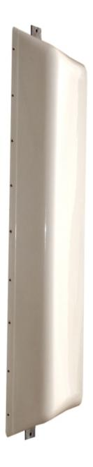
Broadband eight dipole panel covering the 698-806 MHz spectrum. The radiating elements and structural dipoles are entirely welded to the support spine. This results in an enhanced reduction in PIM, even after many years of being in service.
